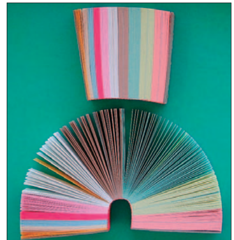
Fig. 11a A book of multi-coloured leaves which can be selectively used as a leaf gauge (Panadent Corp., CA, USA)
